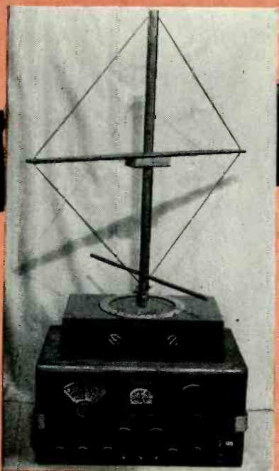
Over-all view of receiving loop. Besides the handle for rotating loop, base has two controls on panel—resonating and impedance matching. A two-turn loop should be used if broadcast band reception is desired.
