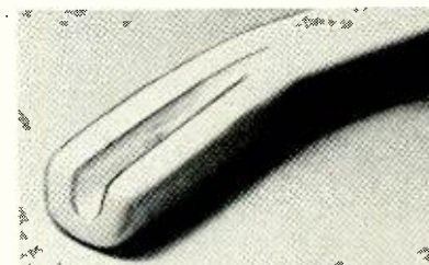
Fig. 16. A groove is filed and gouged in wood arm to accommodate cartridge.
