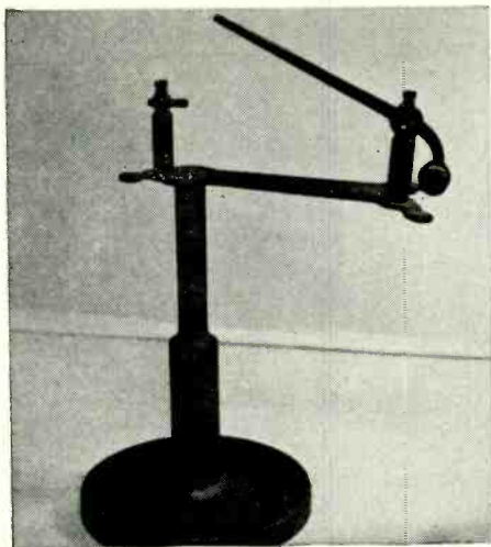
Fig. 1. This device was used to check the speed of record turntables in the heyday of the 78 rpm disc. See Fig. 2 on its use.
