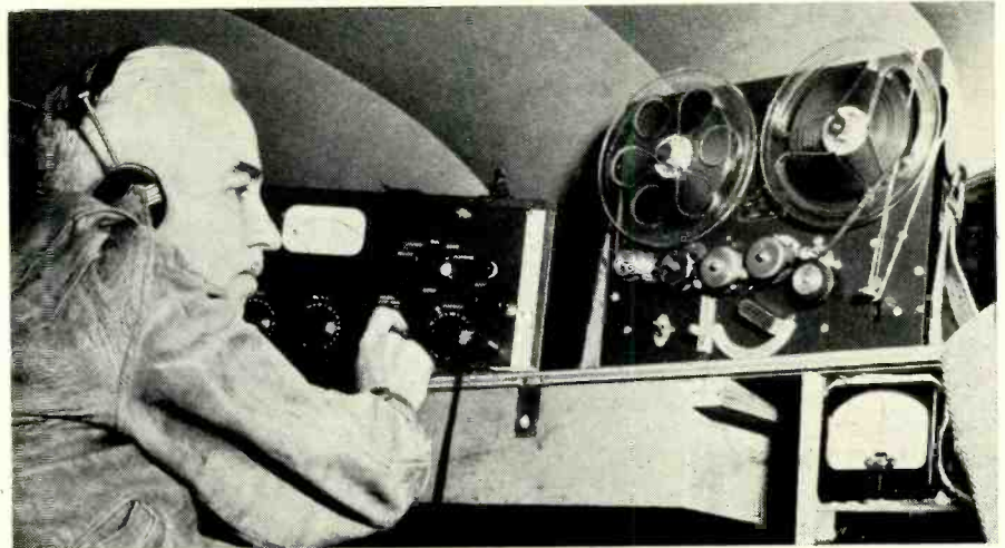
There is no room for back-seat drivers in Prof. Kellogg's "hunting car" where nature's sounds are piped in to the Presto PT-900 tape recorder shown at top right. Other equipment includes volume amplifier (left) and frequency controls at right.
