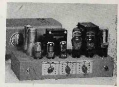
$\pm 1 \frac{1}{2}$  db. Negative feedback and r-c coupling is used. A choice of high or low impedance input is optional, while the output impedances are 4, 8, 250 and 500 ohms. Mark Simpson Mig. Co., 186 W. 4th St., New York 14, N. Y.— RADIO & Television RETAILING
