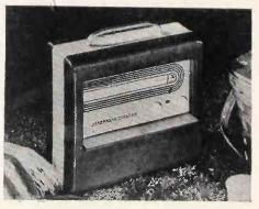
To meet today's vacationist demand, Strom berg-Carlson introduces this "Vagabond" 3way portable. The set comes in 2-color leatherfinish fabric, a 6-tube superhet with 51/2" Alnico PM speaker, tuned r-f, built-in loop. It weighs 15 lbs. and measures 111/2" by 13" by
