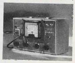
is reversible on 6 d-c voltage ranges covering up to 1200 volts at 51 megohms input resistance, and 6 additional ranges covering up to 3,000 volts at 126 megohms input resistance. 3 db ranges are provided, while 6 ohm scales cover up to 2,000 megohms. McMurdo Silver Co., 1240 Main St., Hartford 3, Conn.— RADIO & Television RETAILING.
