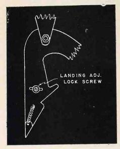
Raise tone arm of Zenith models to remove lift pin, before loosening lock screw.
