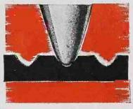
Permanent Sapphire Stylus rides the walls of the record groove, instead of digging into the bottom. Finer tone—virtually eliminates wear and tear.
