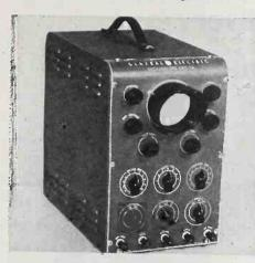
a flat response up to 30 kc, dropping 1 db for each 10 kc thereafter up to 100 kc, resulting in a sensitivity of .3 volt per inch deflection in the range up to 30 kc. General Electric Co., Electronic Dept., Schenectady, N. Y.—RADIO & Television RETAILING
