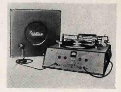
dynamically balanced. Drive shaft of hardened steel revolving on single steel ball. Instantaneous locking lever, speed shift from 78 to 33 1/3 RPM; directional of cut optional at will—lines per inch variable from 90 to 130 with calibrated indicator. Amplifier has phase inversion inverse feedback and tone equalization: 12" PM speaker. Ellinwood Industries, 150 W. Slauson Ave., Los Angeles 3, Calif.—RADIO & Television RETAILING
