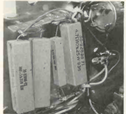
The B+ regulator transistor heat sink, on which the conveniently grouped voltage divider resistors are also mounted.
