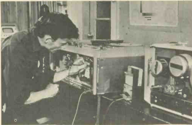
Bench servicing of a video tape recorder in the electronic service facility located in a "penthouse" atop the hospital.
