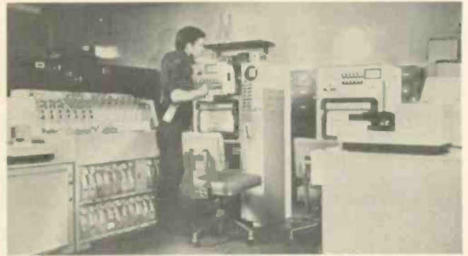
Maintenance of the medical laboratory electronic equipment is also a responsibility of the two electronic technicians employed full time by St. Rita's. Jim Marshall is shown here testing a 12-channel blood analyzer in the medical laboratory.
