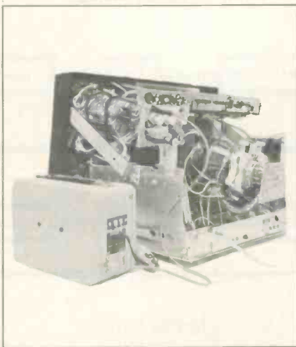
Rear view of Tuner-Mate and Sylvania small-screen color TV receiver showing interconnections for VHF tuner substitution.
