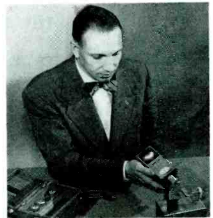
Experimental grid-dip oscillator built around a single 2N33 point-contact transistor, and powered by a miniature 22½-volt hearing aid battery. The device, developed as a private project by Clarence A. West, an amateur (W21YG, Roselle, N. J.), is used to determine the resonant frequencies of tuned circuits. The complete unit, together with power supply, is contained within a metal case measuring 5" high, 2¼" wide, and 2¼" deep. Instrument's power consumption is 25 milliwatts. (Courtesy RCA.)
