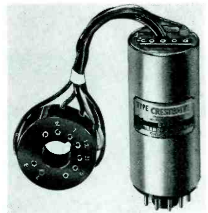
A multi-use video tube brightener and rejuvenator, that operates with either series or parallel connected picture tube filaments, and can be used to isolate the tube filament or to increase tube filament voltage or both, via a simple switching device. (Crestrite; Crest Transformer Corp.)
