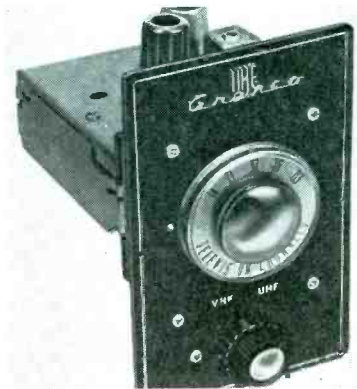
Two cavity front end for all-channel reception, which may be powered from TV chassis; vhf channels 5-6 are used as if. Input is 300 ohms with high output impedance. Power requirements are B+ 100-130 volts at 20 ma; filaments 6.3 volts at 450 ma. Supplied with a 6AF4 uhf oscillator and IN82 diode; if amplifier not included. (Model UJ6; Granco Products, Inc., 36-17 20 Ave., L. I. City 5, N. Y.)
