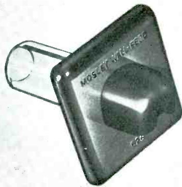
Transmission line wall entrance for house and trailer use which will accommodate either flat or tubular line and will, it is said, seal out rain and snow. Wall-feed permits entrance of wire directly under the eave into the attic. A neoprene gasket is supplied with each unit. (No. 626; Mosley Electronics, Inc., 8622 St. Charles Rock Road, St. Louis, Mo.)
