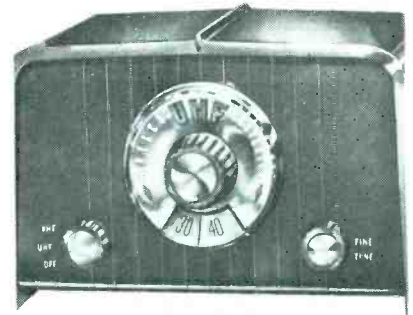
Turret-tune uhf converter, featuring turret-type band-spread tuning unit with a double tuned preselector. Tuning unit is said to have a constant lc ratio. A balanced line oscillator is claimed to keep frequency drift to a minimum. Input antenna terminals are provided for separate uhf and vhf antennas, but can also be used with combination antennas. (Imperial; Walsco Electronics Corp., 3225 Exposition Place, Los Angeles 18, Calif.)
