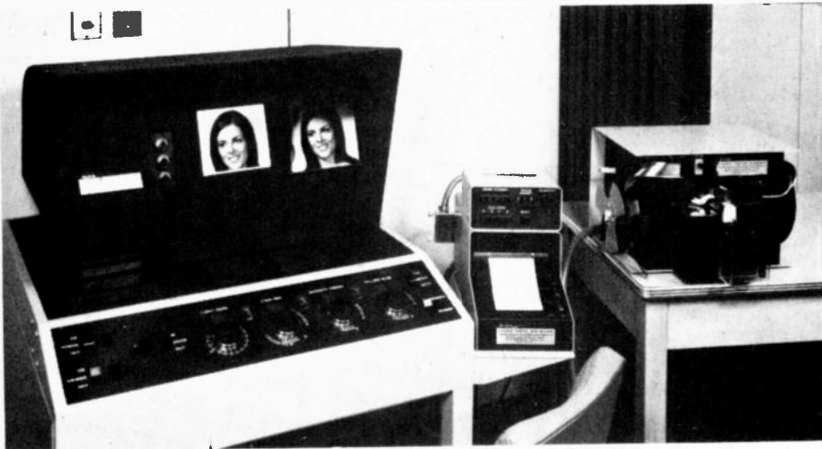
Professional equipment used by color labs includes this Kodak Video Color Negative Analyzer. It uses a 5-in. color TV screen to assist an operator in selecting the correct filter.
