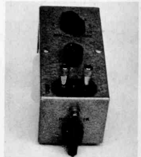
Looking at FRAG from the front shows the frequency range selector, as well as the output terminals and level controls on top.
