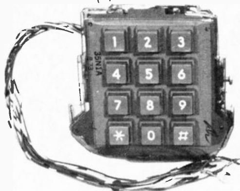
This is what you can get from the surplus dealers: a Western Electric Touch-Tone pad and plastic housing.
