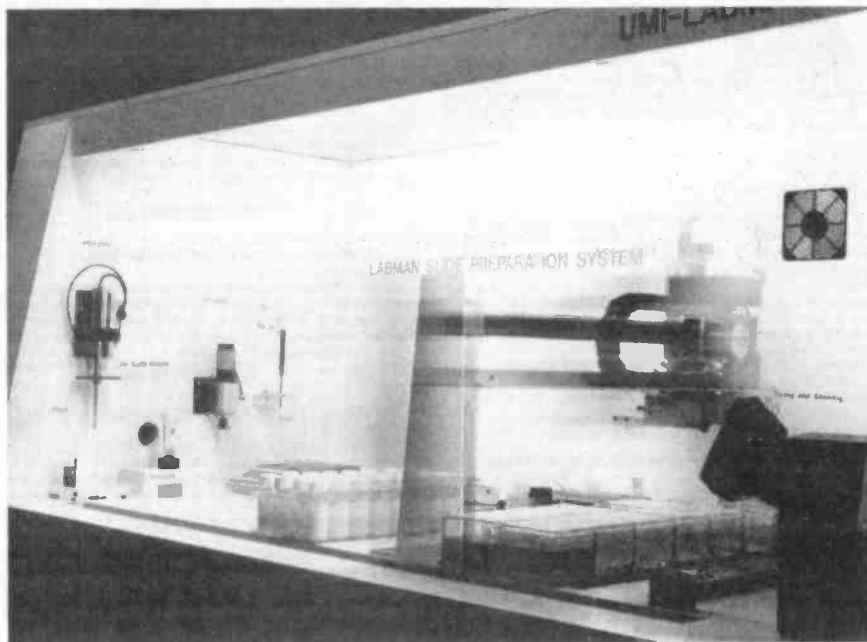
A Labman 900 set up with a Bar Code reader as a slide preparation system
