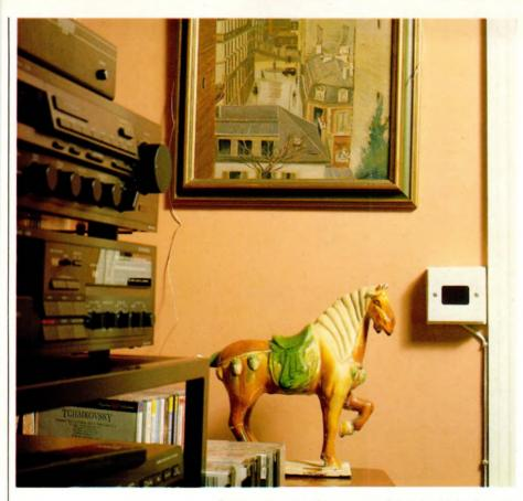
QED's woll-mounted transmitter (above), which relays the infra-red sensors' commands back to the equipment. Below: Not being antique the hi-fi is tucked uway under a staircase.
