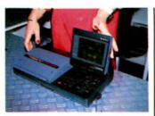
Above: the 'laptop video' from Hitachi uses full-size VHS tapes and flip-up LCD screen.
