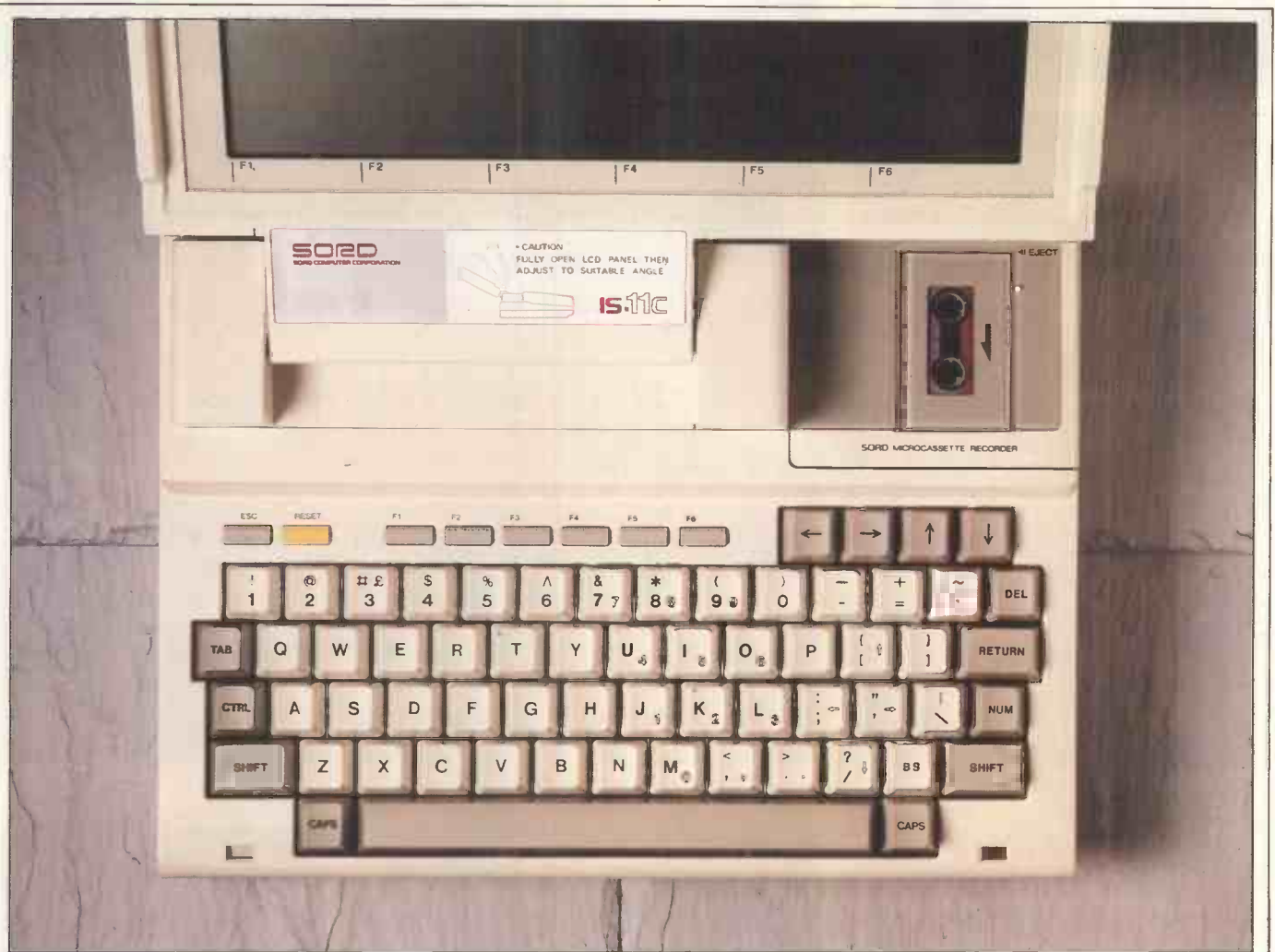
The keyboard comprises 62 full-stroke keys and eight calculator-type keys, including six function keys
