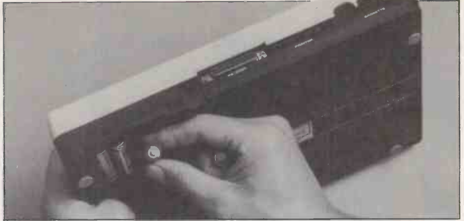
Four AA batteries power the Tandy 100, with rechargeable back-up to maintain RAM.
