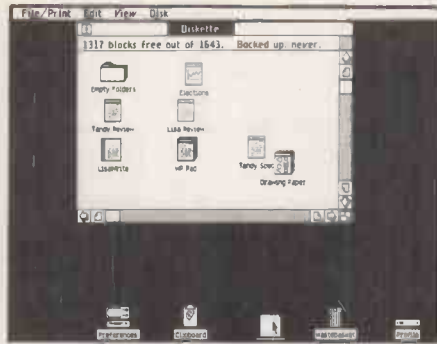
Figure 2. Moving the pointer over the diskette icon with the mouse and clicking it opens up the diskette icon into a window revealing what is on the diskette.
