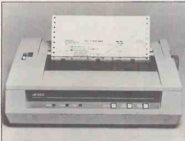
The LA-50 is a typical modern dot-matrix printer which can produce a variety of type styles with a seven by nine matrix, plus bit-map dot-addressable graphics. It prints at 100cps bidirectionally. In the enhanced typeface it overprints to provide a 13-by-nine dot character at 50 cps. It has both tractor and friction feed and can handle fan-fold, single sheets and rolls of paper. The LA-50 is from DEC but can be supplied for most small micros by Rapid Terminals, Rapid Recall Ltd, Rapid House, Denmark Street, High Wycombe, Buckinghamshire HP11 2ER.
