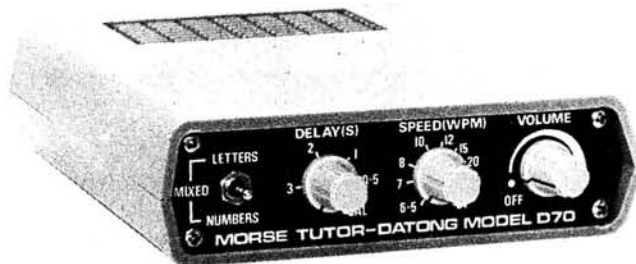
Fig. 3: One of the new random Morse generators for self-tuition
