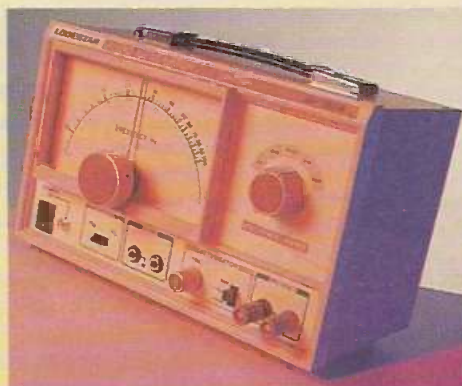
AG2601 is a portable mains-powered instrument covering 10Hz to 1MHz in five overlapping decades. Sinewave distortion between 500Hz and 50kHz is just 0.05%.
