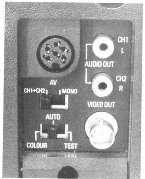
The rear panel features a useful AV plug that brings together all video and audio signals.
