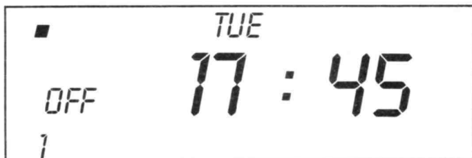
The 'stop time' prompt. Start time is now displayed as the base.
