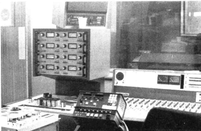
The main 8-track desk with metering and panel controls.
