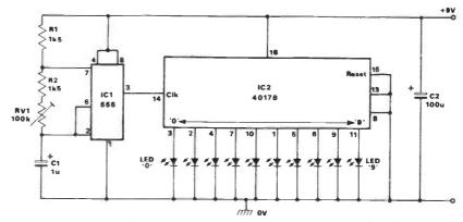
Fig 3 10-LED chaser or sequencer can be used with <9V supply
