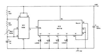
Fig 8 4-LED continuous 'moving dot' display
