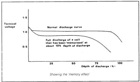
can be overcome with little damage to the cell by giving it a deep discharge.
