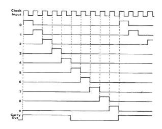
Fig 2 Waveform timing diagram of the 4017B
