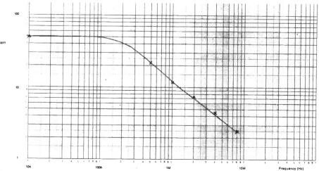
Fig 2 Frequency response of simple amplifier
