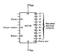
Fig 1b Diagram and data for the 4017B
