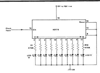
Fig 4 This version of the 10-LED chaser can be used with supplies ≤15V
