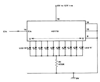
Fig 5 This version of the chaser can be used with supplies ≤12V
