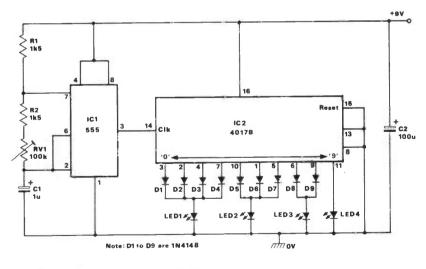
Fig 11 4-LED continuous 'accelerator' display
