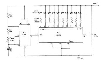
Fig 7 10-LED moving hole display
