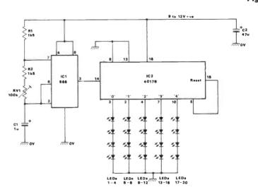
Fig 14 This 4-bank 5-step 20-LED chaser must be used with a supply >9V
