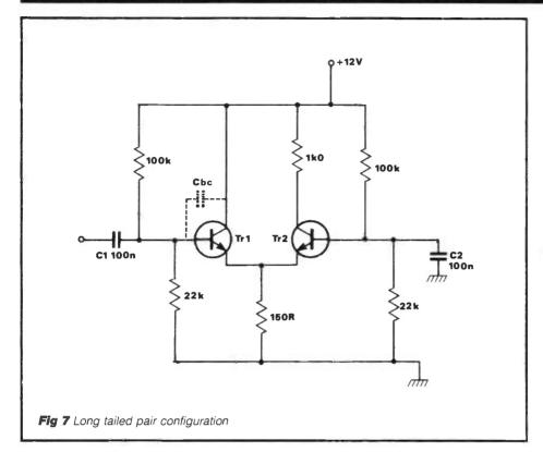
So for le at 2mA,  $f_T$  at 300MHz, Cbe is 42pF – quite significant at even low RF.
