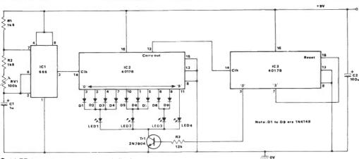
Fig 12 4-LED intermittent 'accelerator' display
