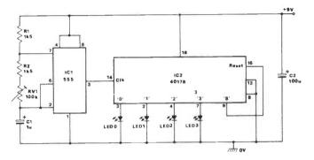
Fig 9 4-LED intermittent 'moving dot' display with 50% 'blank' period
