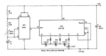
Fig 10 Circuit of a 4-LED 5-step sequential turn-off display
