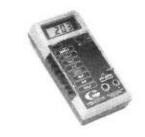
GSC has introduced the Model 3000 digital capacitance meter, a precision test instrument designed for handheld battery operation.
