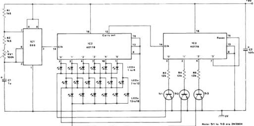
Fig 13 Multiplexed 6-LED x 3-line moving dot display
