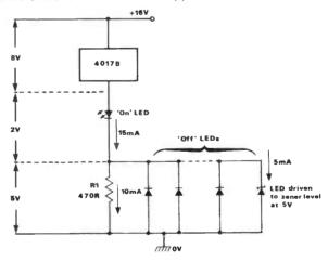
Fig 6 Possible equivalent of the Fig 5 circuit with a 15V supply
