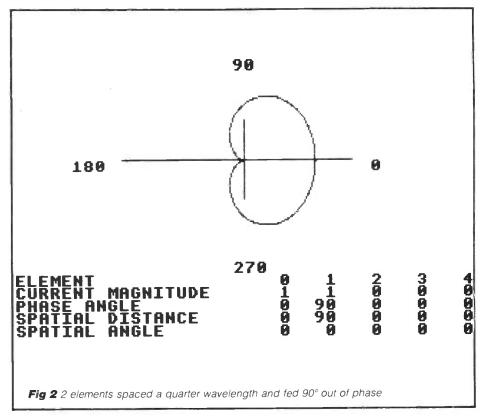
of 90 degrees. The two elements are spaced one quarter of a wavelength apart. (This is a common textbook example.)
