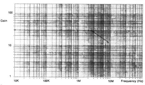
Fig 6 Cascode frequency response
