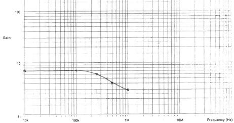
Fig 13 FET amplifier frequency response
