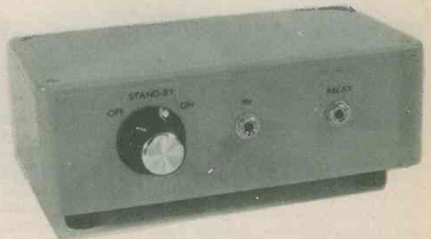
The alarm unit is housed in a small plastic case which can be easily concealed. The photocell then couples to the input jack socket via screened cable
