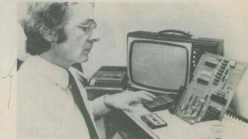
G. R. Electronics add Video Board and Pocket Terminal to Commodore's KIM1 Microprocessor, using a domestic TV as visual display unit
