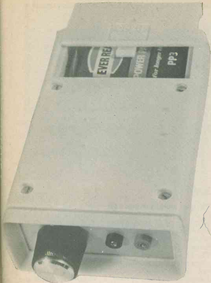
The case specified has a compartment which accommodates a PP3 battery
