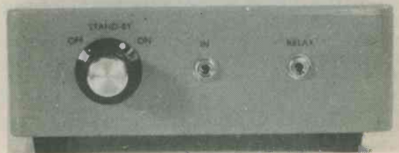
The front panel of the light change alarm carries the Set-Reset switch and jack sockets for connection to the photoconductive cell and the external alarm circuitry
