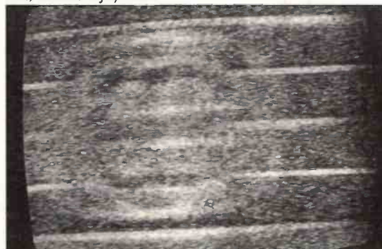
Fig. 2: Typical reception via F2-layer propagation. This was Thailand received on Channel E2 by Pertti Salonen in Finland.
