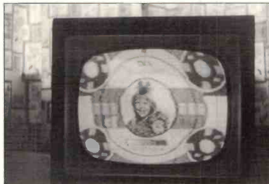
Fig. 1: Garry Smith's first DX season using a modified Bush TV56 receiver and indoor dipole. The set is displaying a Swedish test card, received in July 1969.
