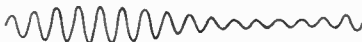
Fig. 2. Simplest amplitude modulation of Fig. 1, in which the modulating waveform itself is a pure sine of lower frequency.
