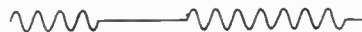
Fig. 3. Sample of carrier wave interrupted by morse keying. Here the carrier cycles that remain are identical with those in Fig. 1, so where do side frequencies come in?
