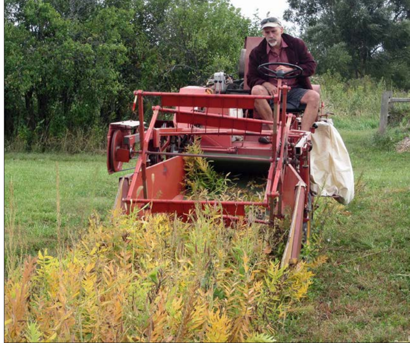
Combining butterfly milkweed with a Hege 125B, 1978 model plot combine. (Photo: Tallgrass Prairie Center, University of Northern Iowa.)
