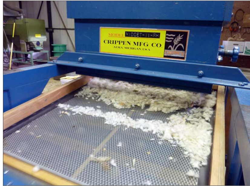
Milkweed material moving across the top screen of an air-screen cleaner. Seed will fall through the holes in the screen and the floss and other debris that travels across the screen will be discarded. (Photo: Brianna Borders, The Xerces Society.)
