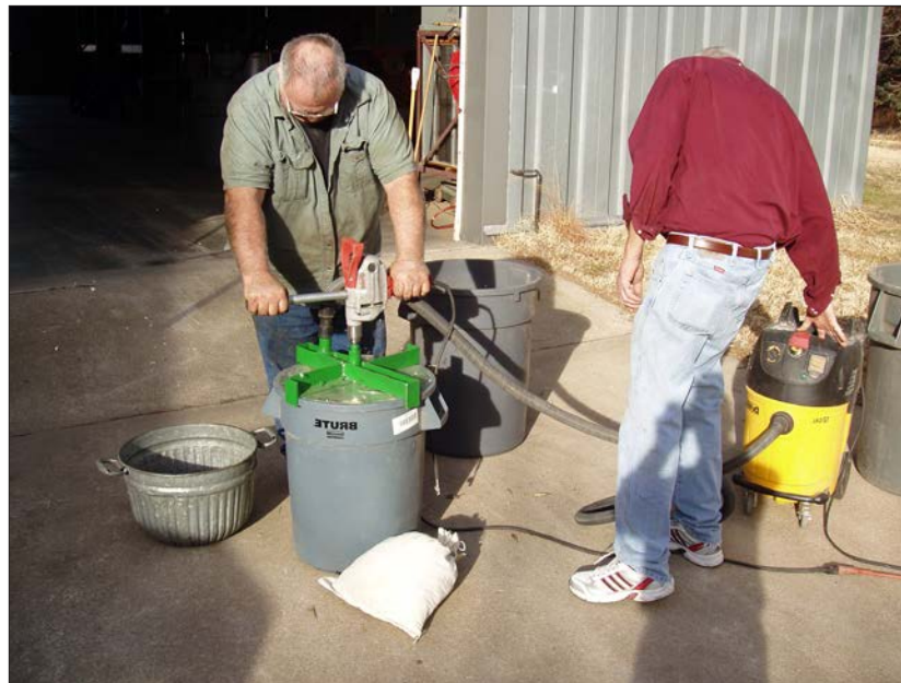
Clockwise from top left: Milkweed seed separator constructed by the USDA-NRCS Plant Materials Center in Manhattan, Kansas. USDA-NRCS staff operating a milkweed seed separator at the Manhattan, Kansas Plant Materials Center. (Photos: USDA-NRCS Manhattan Plant Materials Center.)
