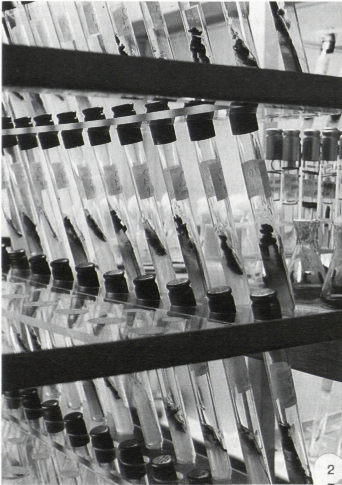
Fig. 2: Shelves made of acryl-glass to enable light diffusion within the racks.
