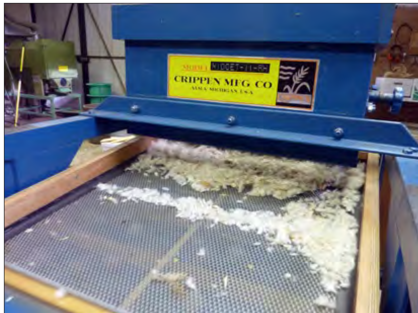
FIGURE 6.22: Plant material moving across the top screen of an air-screen cleaner. Seed will fall through the holes in the screen and the fluff and other debris that travels across the screen will be discarded.
