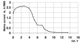
Figure 4.10 Input current under resistive load voltage variation
