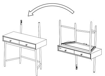
2. Attach the left leg(B) and right leg(C) onto the back side of the drawer box unit(A) using 2pcs M6\*30 bolt (F) as shown below.
