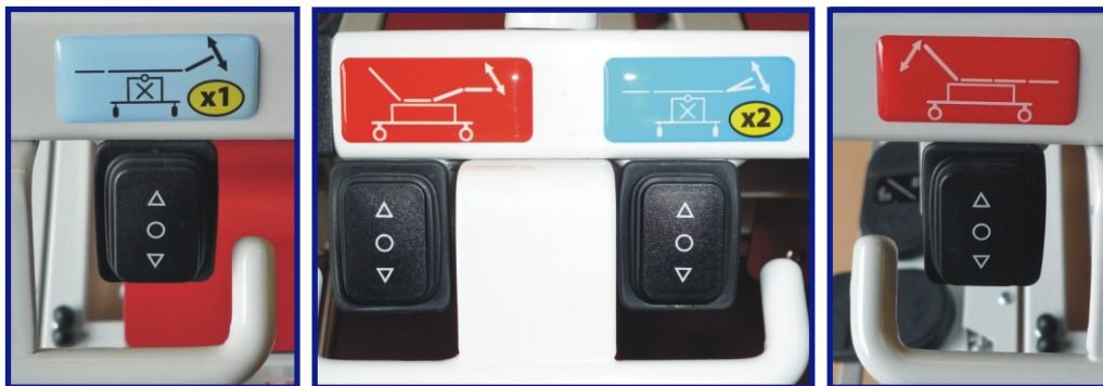
The pictures above illustrate the hand-operated side controls of the bed (see text for detail). Note the protective guards designed to prevent accidental activation of a switch during patient turning or care delivery.
