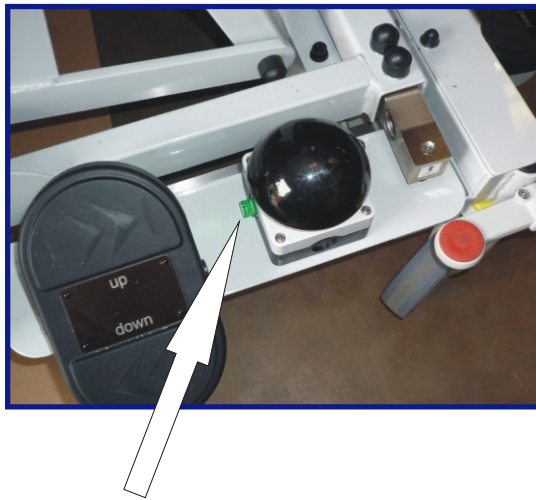
This picture shows the additional foot operated power cut-off button (see text above). Power indicator light shown by arrow - particularly useful in low light conditions.
